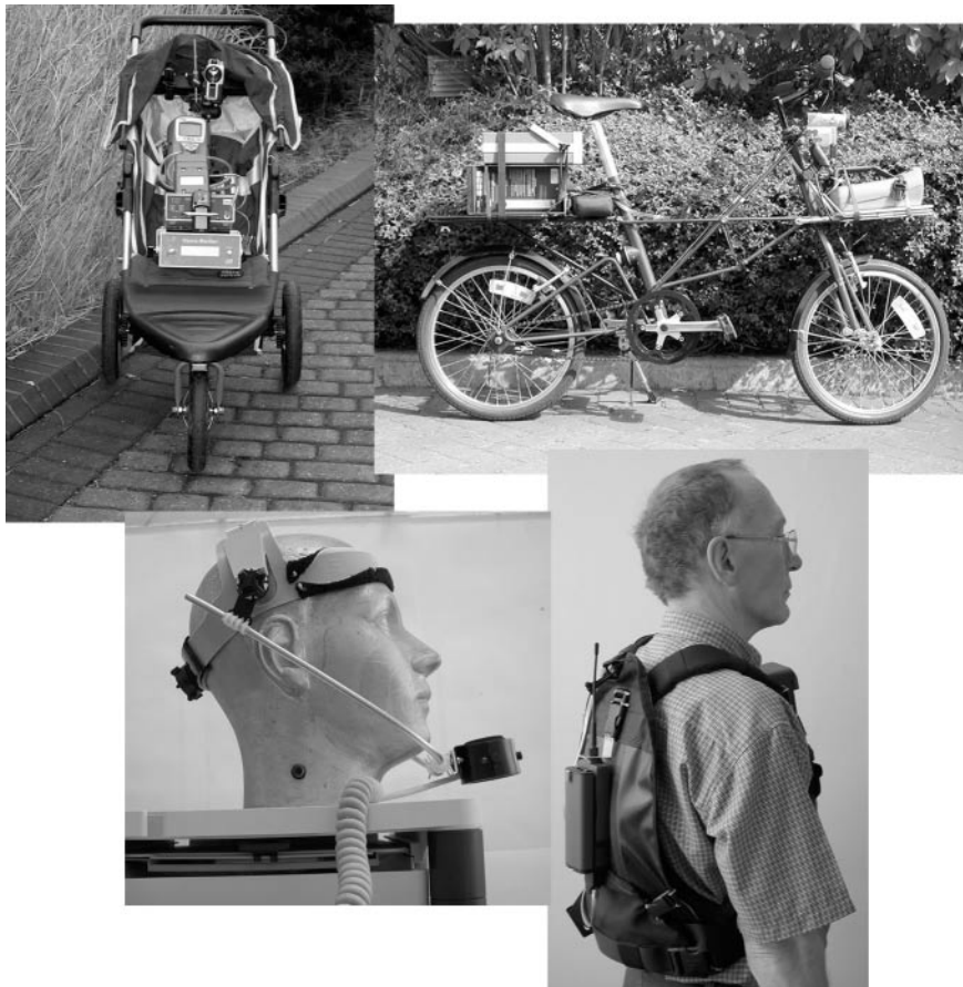
Fig. 4. Examples of instrument mounts for VEM: general purpose backpack, headset for solder fume monitoring, pushchair and pedal cycle for environmental monitoring.
