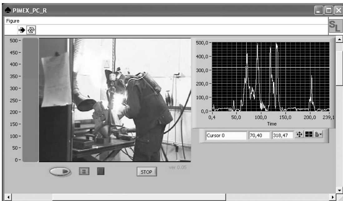
Fig. 1. Example from a PIMEX-PC recording. The video picture window shows a person welding and carrying a monitoring instrument for fume in a backpack. The graph window to the right shows how the welder's exposure to welding smoke has varied during the period. The bar graph to the left shows the instantaneous exposure level.
